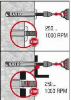
Drive the anchor rod with the setting tool (see Table B3) into the hole, applying moderate pressure and with the hammering action switched on (250 RPM to maximum 1000 RPM).
