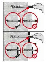
Check the setting depth with the marked element.
