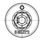
Marking 1: Steel element type, size and fixture thickness; e.g., HAS-TZ M12/50
