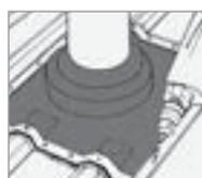
6. Fix to the middle front and middle back of the Dektite® and fix progressively towards the edge.
