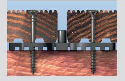
Furthermore, it guarantees spaces between the boards and support rails required for good ventilation. This ensures that any waterlogging that may have occurred can dry out. About 15 – 20 pieces are needed per m<sup>2</sup>, depending on board width.
