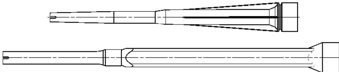
**Injection adapter and Extension tube for static mixer**
