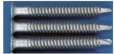
Fig. 20: Screws with highly corrosion-resistant multilayer coating after 15 cycles of the sulfur dioxide corrosion test (showing no corrosion).
