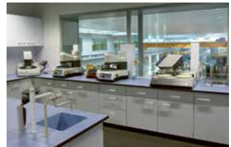
Fig. 23: Metallographic laboratory equipment (grinding and polishing).
