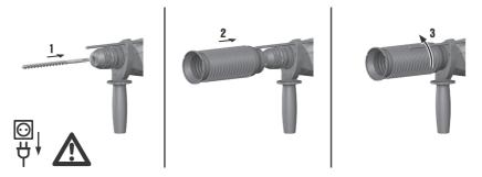
▶ Fit the DCD dust collection module for overhead work.
