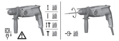
Set the function selector switch to the "Drilling without hammering action" position
