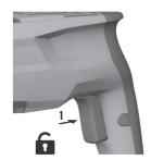
Press and lock the control switch.
