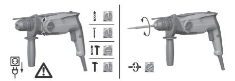
► Set the function selector switch to the "Drilling with hammering action" (hammer drilling) position (↑).
