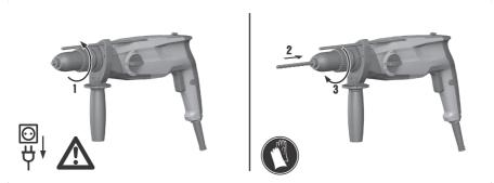
Fit the drill bit or other accessory in the three-jaw chuck or, respectively, remove it.
