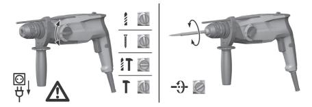
lacktriangle Set the function selector switch to the "Drilling without hammering action" position  $\mspace{1mu}{2}$  .
